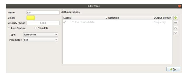
On the left side, additional trace parameters can be changed, while the right side of the window handles math operations that will be applied to the trace data. The available trace parameters are:
