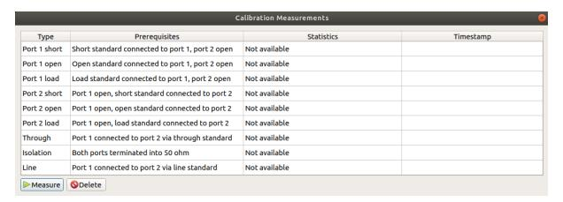
To take a measurement, select the corresponding line and press Measure].
