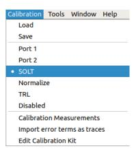
Alternatively, the calibration can be activated by choosing "SOLT" in the toolbar and enabling the calibration checkbox:
