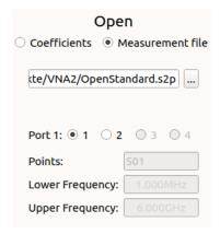
A touchstone file with the measurements is required. If the file contains data from more ports than required (for open, short and load 1-port measurements are needed, for the through 2-port measurements), the correct port(s) has to be selected. If any standard is defined by a measurement, the usable frequency range of the calibration kit is limited to the smallest common range of all measurement.
