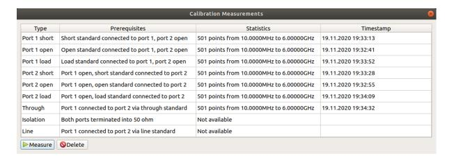
4. Close the "Calibration Measurements" window and activate the SOLT calibration by selecting Calibration SOLT:
