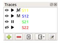
The list shows all available traces, by default the four S parameters S11, S12, S21 and S22. Different icons in front of the trace names indicate the state of the trace. Clicking on one of the icons toggles the state:
