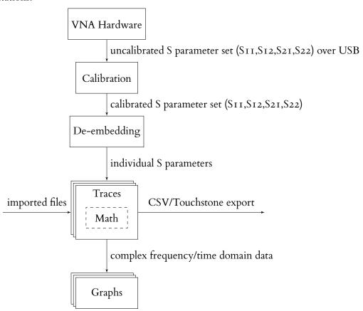
The central element of the signal flow is the concept of **traces**. A trace is created from a single S parameter across frequency (either measured by the LibreVNA or imported from an external file). Once the data is captured in a trace, optional math operations may be applied to it (e.g. performing a TDR to transform the data into the time domain) and the result of these operations are passed on to the graphs.
