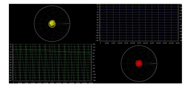
3. Select Calibration Calibration Measurements and take the required measurements. In this case, the measurement "Isolation" (optional for SOLT) has not been taken, as well as the "Line" measurement (not required for SOLT)
