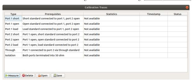
To take a calibration measurement select the corresponding line in the table, setup the device ports as described under prerequisites and press Measure. Likewise, a measurement can be removed by selecting it and pressing Delete.
