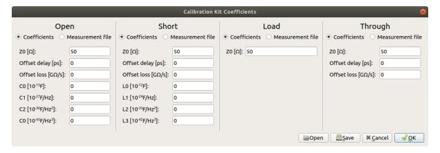
Each calibration standard can either be defined through its coefficients or by measured data from a Touchstone file. The calibration kit data is stored together with the calibration data when saving it in the Calibration Data Dialog.
