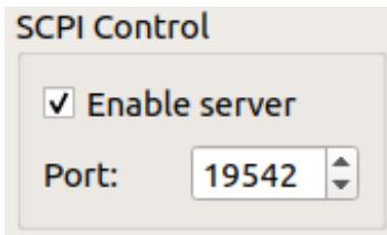
If enabled, it will accept any TCP connection at the configured port. Once the connection is established, it can be used to send SCPI commands and receive replies. Only one connection at a time is possible, if a second connection is created, the first one will be closed by the LibreVNA-GUI. Alternatively, a port can be manually configured by setting the “port” argument:
