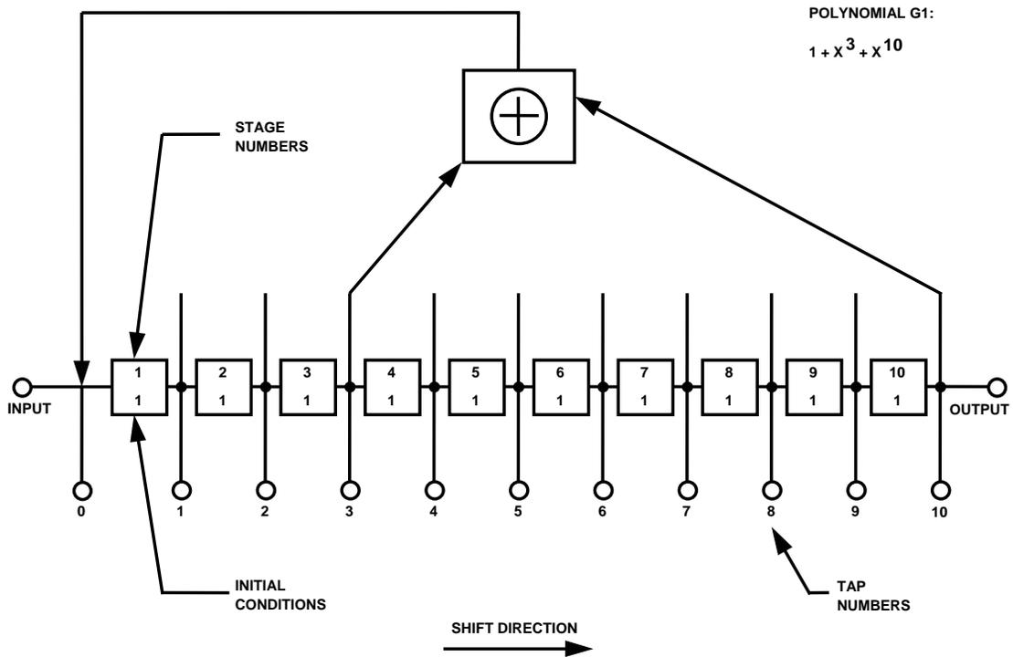
Figure 3-8. G1 Shift Register Generator Configuration
