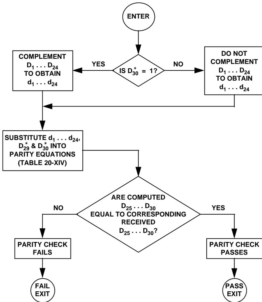
Figure 20-5. Example Flow Chart for User Implementation of Parity Algorithm
