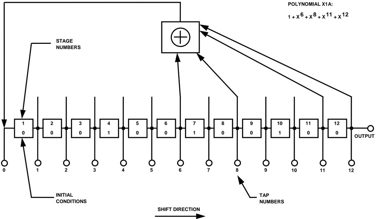
Figure 3-2. X1A Shift Register Generator Configuration
