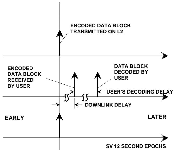
Figure 3-15. Convolutional Transmit/Decoding Timing Relationships
