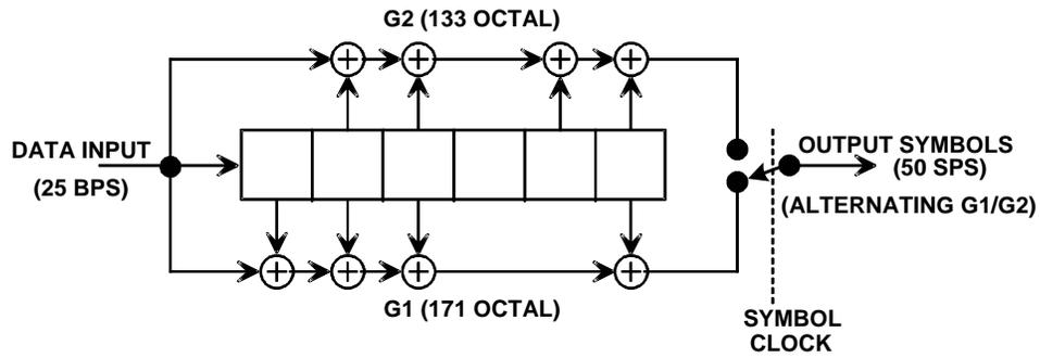
Figure 3-14. Convolutional Encoder
