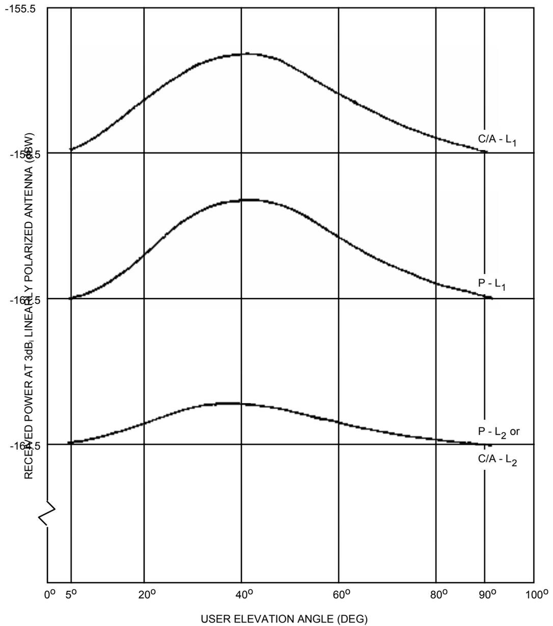
Figure 6-1. User Received Minimum Signal Level Variations (Example, Block II/IIA/IIR)
