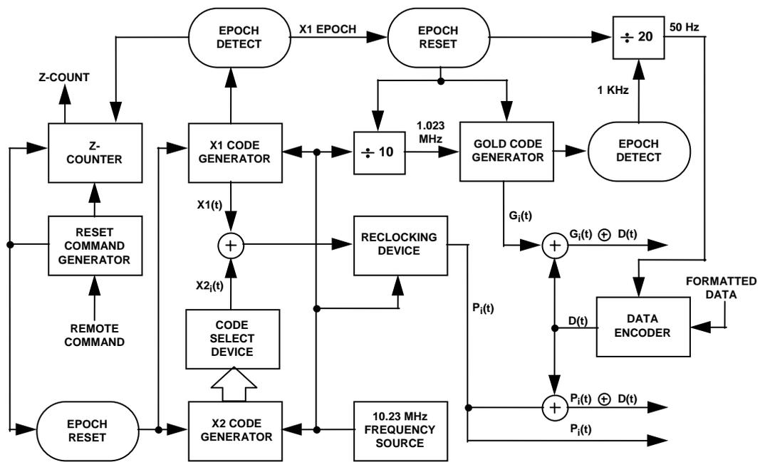
Figure 3-1. Generation of P-, C/A-Codes and Modulating Signals
